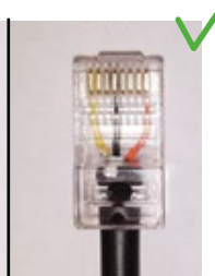
Correct wiring of the RJ45 plug for G-Motion units.
